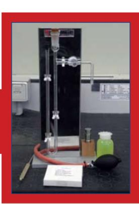
This apparatus is used to determine the fineness of Portland cement in terms of the specific surface expressed as total surface area in square centimeters per gram of cement.
