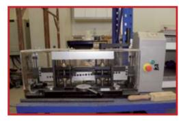
BAR TRACING MACHINE FD55/S Marking of steel bars for the determination of elongation (%)
